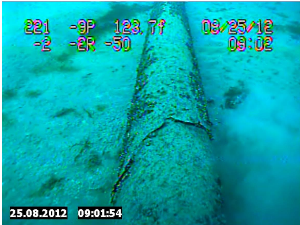
Figure 9. Photo Clipped from Enbridge 2012 Underwater Inspection Video of the East Line Taken on 8/25/2012 at 09:01:54 Showing Missing and Disbonded Coating
